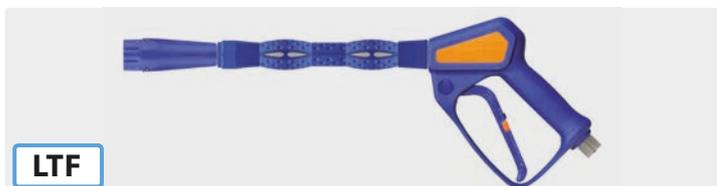
Foam lance with **easywash365+** gun weep version, lance with extension ST-9.1 245 mm and foam head ST-75. Max. 310 bar / 25 l/min / 150 °C
