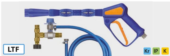
**easywash365+** foam set: **easywash365+** foam lance standard with foam head ST-75, injector ST-160 (M22 F and 2 x M22 M) with metering valve ST-161, suction hose 1,000 mm and suction filter ST-32. Max. 310 bar / 90 °C
